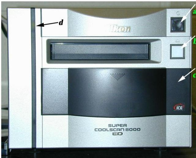
Figure 1. Nikon Super CoolScan 9000 front view. *a.* Mains button; *b.* Eject button *d.* LED
